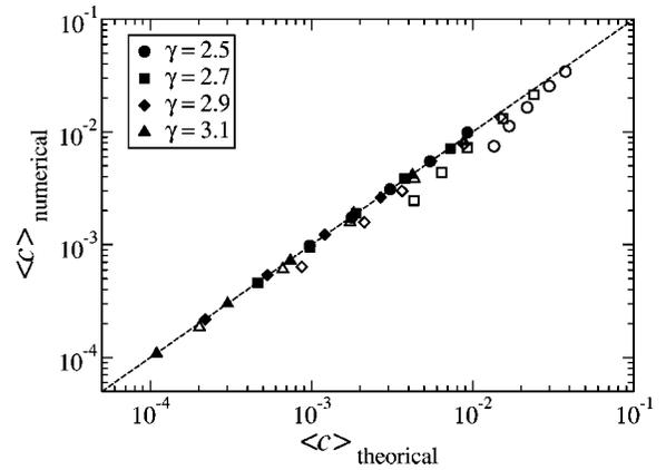
FIG. 3. Numerical average clustering coefficient  $\langle c \rangle$  as a function of the corresponding theoretical value, given by Eq. (5), for the CM (open symbols) and the UCM (solid symbols) algorithms. The different points for each value of  $\gamma$  represent different network sizes  $N=10^3, 3 \times 10^3, 10^4, 3 \times 10^4$ , and  $10^5$ .
