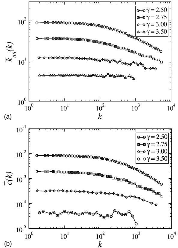
FIG. 1. Average nearest-neighbor degree of vertices of degree  $k$ ,  $\bar{k}_{nn}(k)$  (a), and average clustering coefficient  $\bar{c}(k)$  (b) for the original CM algorithm with different degree exponents  $\gamma$ . Network size is  $N = 10^5$ .
