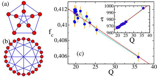
FIG. 3: Cage graphs for  $k = 3$  and (a)  $g = 5$  (Petersen) and (b)  $g = 7$  (McGee). Right panel: Percolation threshold (main) and average first-passage time (inset) as a function of the eigenratio  $Q$ , as obtained during the optimization of a network with 500 nodes and  $\langle k \rangle = 3$ . The initial network corresponds to a 3-regular graph with  $N = 500$ .
