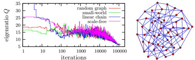
FIG. 1: Eigenvalue ratio,  $Q$  as a function of the number of algorithmic iterations. Starting from different initial conditions, with  $N = 50$ , and  $\langle k \rangle = 4$ , the algorithm converges to networks, as the depicted one, with very similar values of  $Q$ .
